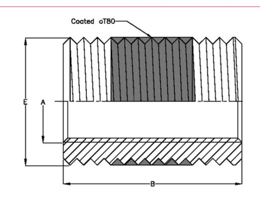
Female thread A = M12Length B= 30Male thread E= M16Type= 97x 000 120.100
